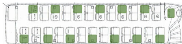
MCI J4500 with typical 56 passenger seat layout following CDC guidelines of social distancing
