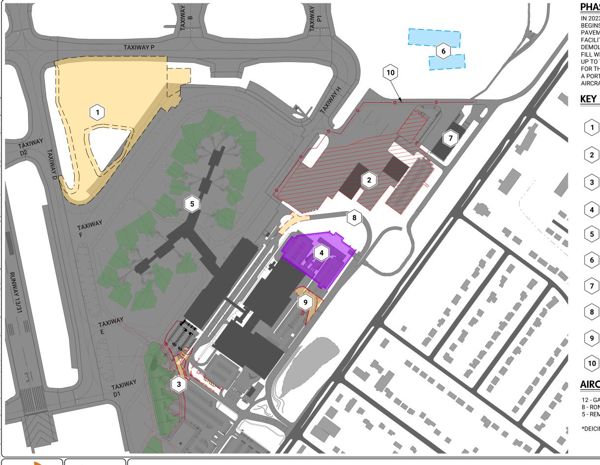
IN 2023 CONSTRUCTION ON THE TERMINAL PROGRAM BEGINS IN EARNEST. EXISTING HANGARS, APRON PAVEMENT, AND PARKING LOTS FOR GENERAL AVIATION FACILITIES IN THE EAST QUADRANT WILL BE DEMOLISHED. APPROXIMATELY 70,000 CY OF EARTH FILL WILL BE IMPORTED TO BRING THE TERMINAL AREA UP TO THE PROPOSED ELEVATIONS. IN PREPARATION FOR THE START OF TERMINAL CONSTRUCTION IN 2024, A PORTION OF THE GREEN LOT WILL BE CONVERTED TO AIRCRAFT PARKING.
