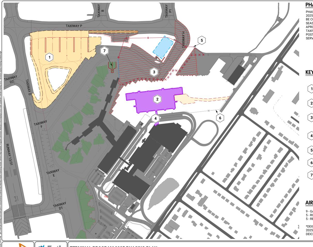
PHASE 1A TERMINAL CONSTRUCTION WILL CONTINUE IN 2025. TERMINAL APRON PHASE 1 - DEICING PADS WILL BE COMPLETE PRIOR TO THE START OF DEICING SEASON, THEN WORK WILL BEGIN ON THE TERMINAL APRON PHASE 2 PROJECT WITH THE DEMOLITION OF TAXIWAY H, AND REMOVAL OF APRON PAVEMENT. POSTIONS C6A AND C7B WILL BE TAKEN OUT OF SERVICE.
