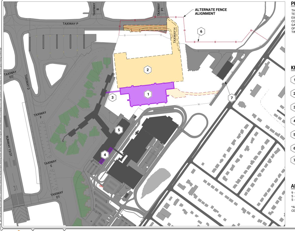
THE 2026 WORK INCLUDES COMPLETION OF THE NEW TERMINAL PHASE 1A, COMPLETION OF CONNECTION TO EXISTING CONCOURSE C FROM THE NEW TERMINAL. COMPLETION OF THE PEDESTRIAN BRIDGE FROM THE GARAGE TO THE NEW TERMINAL. START OF DEMOLITION OF THE EXISTING PROCESSOR BUILDING. COMPLETION TIME FRAMES ARE PROJECTED END OF 3RD QUARTER.
