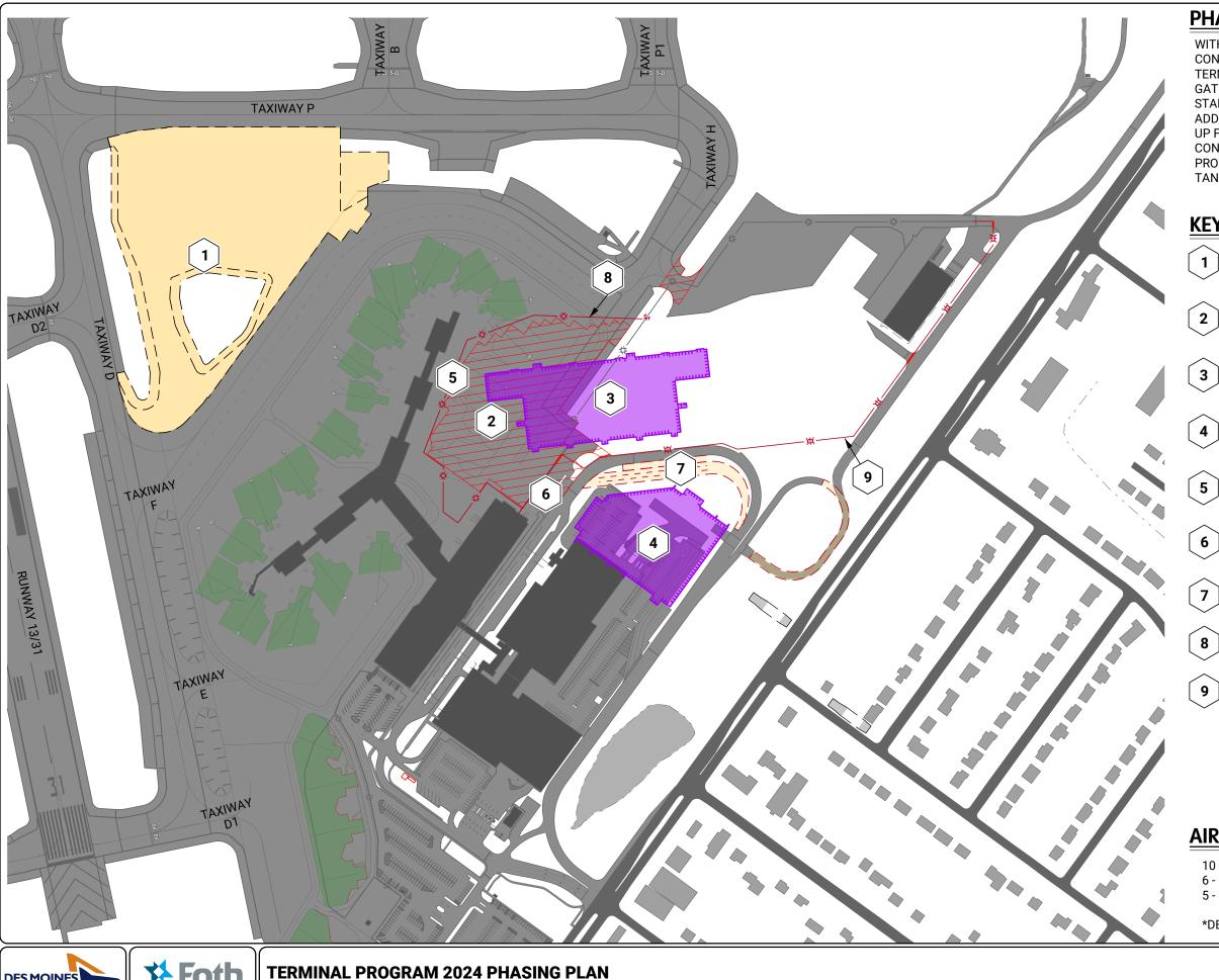
WITH THE START OF TERMINAL BUILDING CONSTRUCTION IN 2024 A PORTION OF THE EXISTING TERMINAL APRON WILL BE DEMOLISHED, REMOVING GATES C2, C4, AND C6B OUT OF SERVICE. PRIOR TO START OF TERMINAL FOUNDATION CONSTRUCTION ADDITIONAL FILL WILL BE REQUIRED TO BRING THE SITE UP FOUR TO EIGHT FEET. DEICING APRON CONSTRUCTION WILL TAKE PLACE, WHICH WILL PROVIDE A NEW DEICING FLUID STORM WATER RUNOFF TANK AND FOUR CENTRALIZED DEICING PADS.
