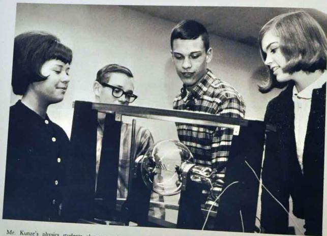
Mr. Kunze's physics students observe an instrument which determines the ratio of charge to mass for an electron.
