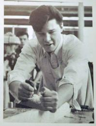
In preparation for sanding and finishing, Greg Lonberger files a plank of wood.
