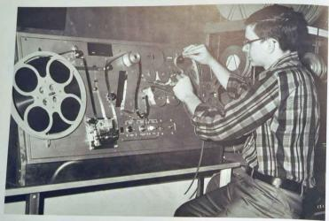
A valuable asset to the visual aids department is the defect detector which cleans tapes and at the same time checks for any damages.
