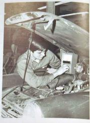
Greg Gordon attempts to diagnose the trouble in an engine during Mr. Seidenfuss' auto class by measuring its rpm's.
