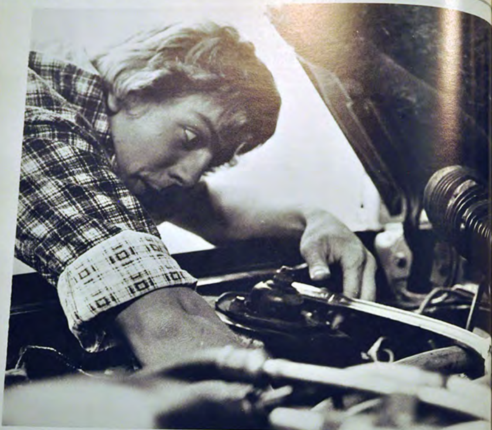
Arm-deep in the engine, senior Bruce Padalik changes a spark plug while attaching a wire to the distributor during his Auto class, where the basics of engine maintenance are learned first-hand.
