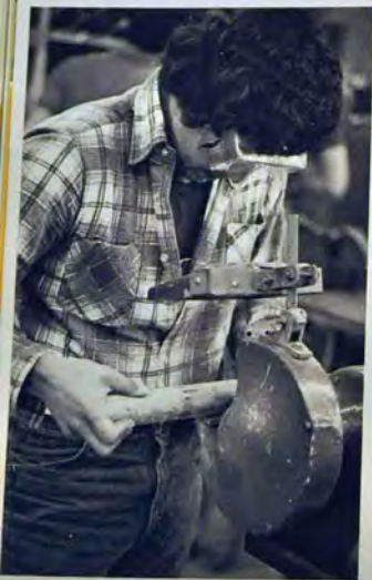
Wire brushing and careful pipe rotation by Jay Carriedo prepare the cylinder for proper fitting. Wearing safety goggles and working under strict safety regulations aid in the prevention of accidents in the metal shop.
