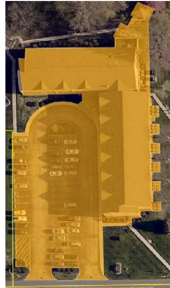
Figure 4-5 Example of Impervious Area Digitized from a Nonresidential Parcel
