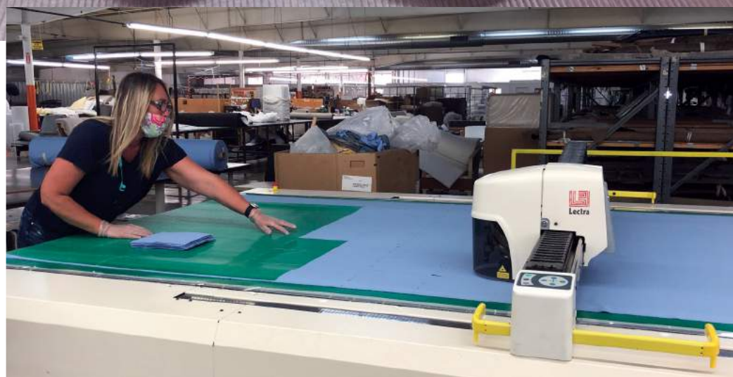
Taylor King and Huntington House fabric cutters use their advanced digital technologies to precisely cut out PPE mask panels ensuring the least amount of fabric waste.
