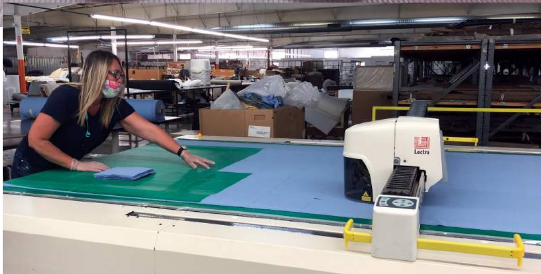
Taylor King and Huntington House fabric cutters use their advanced digital technologies to precisely cut out PPE mask panels ensuring the least amount of fabric waste.
