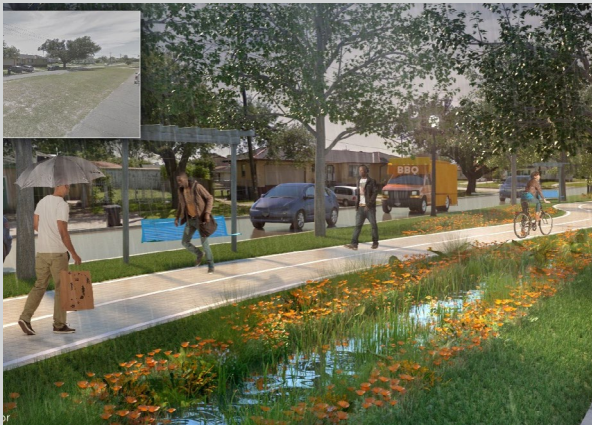
Vegetated swales used for stormwater collection/treatment
