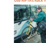
Bicycle racks are attached to the front of all full-sized RIPTA buses (not trolley buses) and are easy to use. There is no additional charge to use the racks. Please alert the driver before you attach your bicycle and then follow the instructions below.
