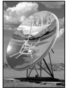
The hourly weather information collected by the RAWS is transmitted through a satellite, back to NIFC, and then distributed to various locations via the internet.
