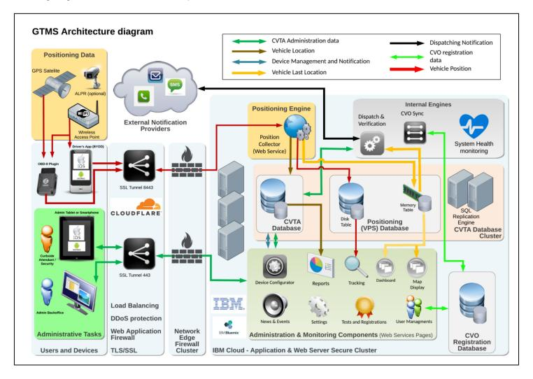
ReserTrac GTMS backend is the collection of cloud-based hosting environments, network interfaces and 3<sup>rd</sup> party services which come together to deliver the full functionality of the previously described components. Each GTMS client receives their own independent GTMS cloud backend – **we do not share cloud resources among clients**.
