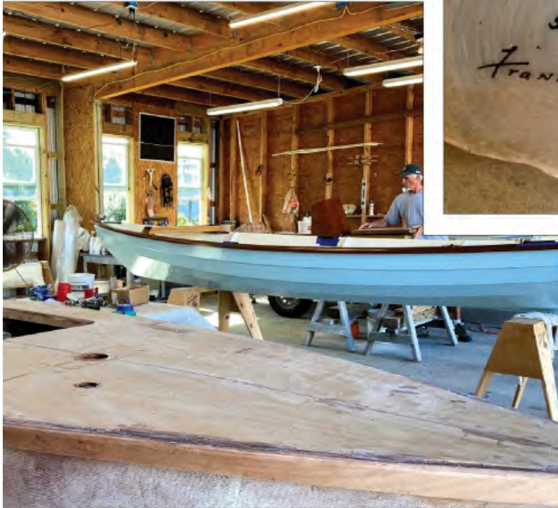
Expanded workshop at Farley Boat Works. Volunteers working on an 18' fly-fishing skiff (foreground) and a 16' sailing dory (middle).
