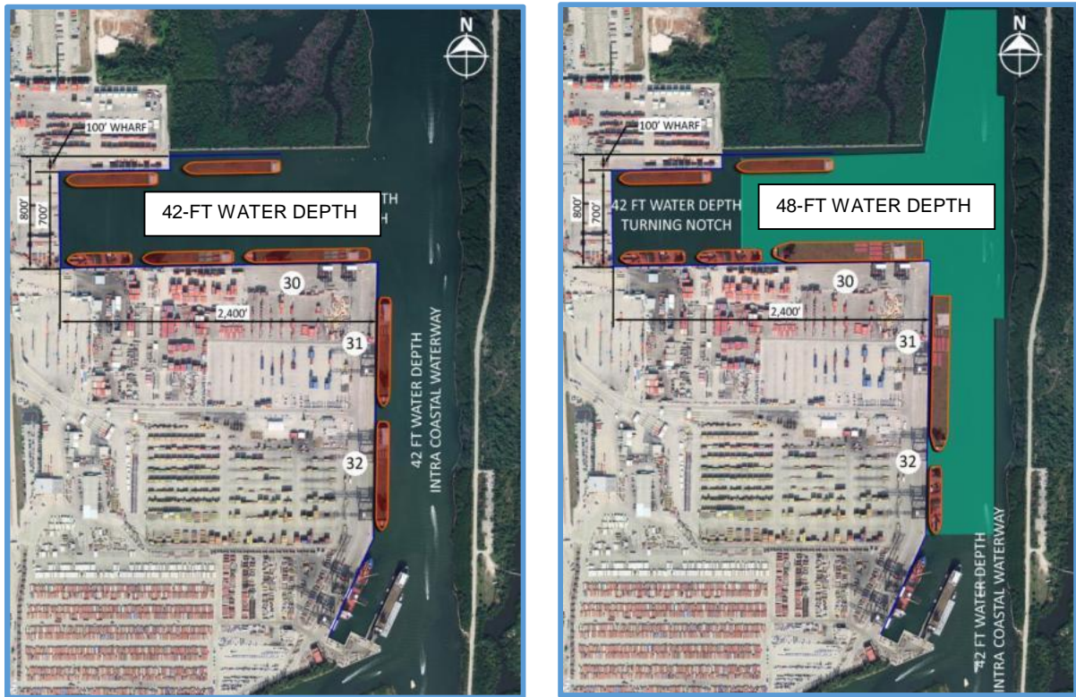
Figure ES-20 SOUTHPORT TURNING NOTCH EXTENSION (AT 42- AND 48-FOOT DEPTHS)
