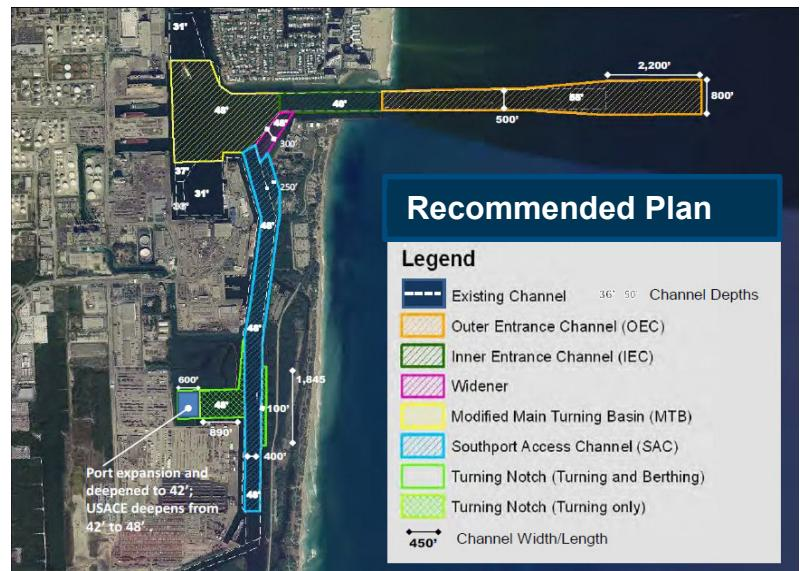
Deepening the east end of the Southport Turning Notch, including a portion of the extension, from 42 feet to 48 feet (plus 1-foot required and 1-foot allowable overdepth for a total of 50 feet) in the area extending 1,300 feet from the SAC, with an additional 100-foot widening parallel to the channel on the eastern edge of the SAC over a length of about 1,845 feet
