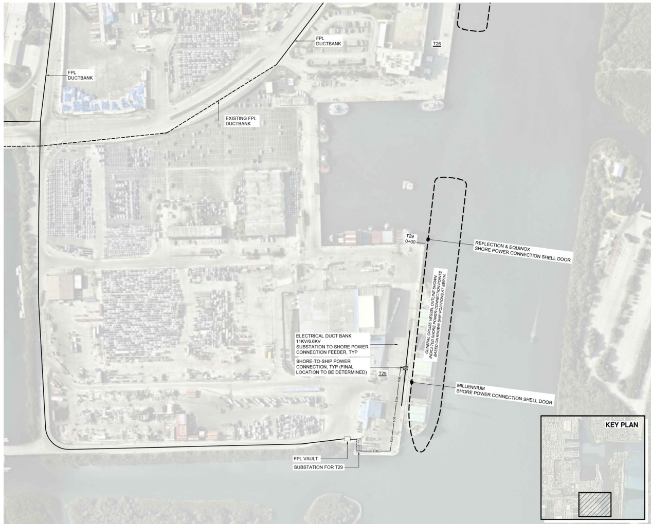
Figure 5-5. CT29 Enlarged Electrical Site Plan (Sheet E114)
