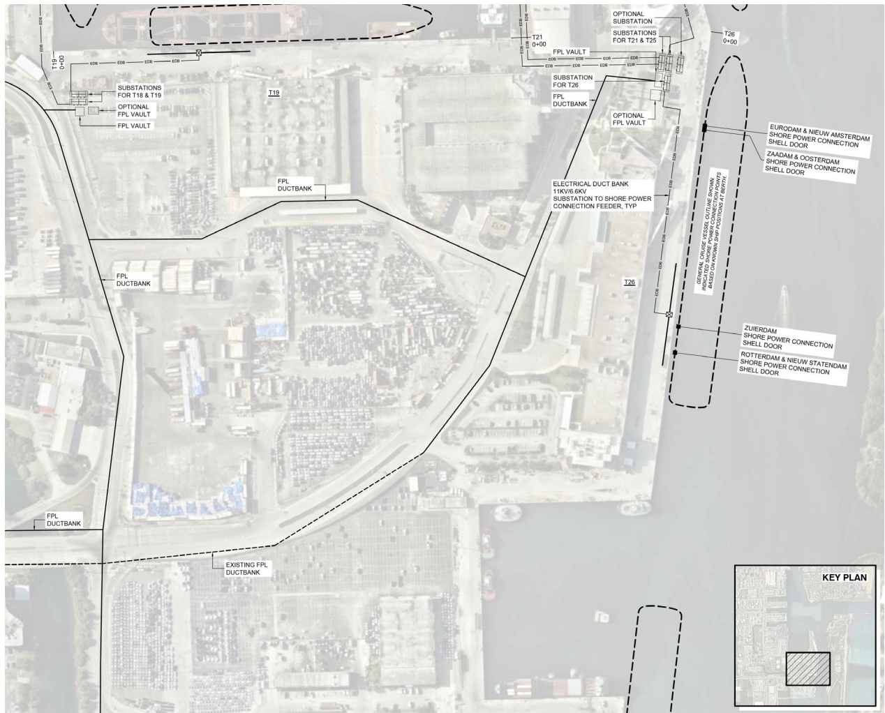
Figure 5-4. CT26 Enlarged Electrical Site Plan (Sheet E113)
