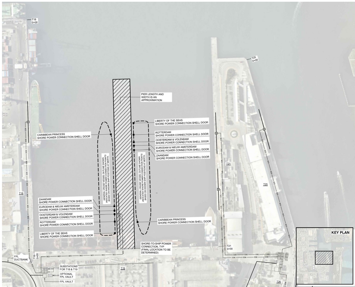
Figure 5-7. Berth 19 Pier Shore Power Option (Sheet 112-A)
