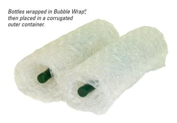
Bubble Wrap® cushioning requires a minimum of 2" of material around sides, top and bottom of bottles. Special attention must be paid to lock Bubble Wrap® securely to contents and add extra void fill when necessary.
