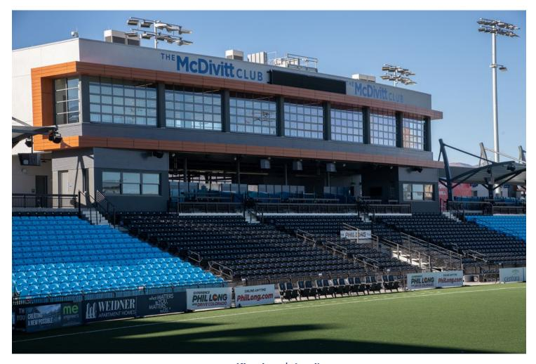
specifications | details Switchbacks Football Club I Colorado Springs, CO Architect: Perkins & Will ABOVE: West Side 15 Rows x 345', Interlock 2000 decking system, 2,456 Seats BELOW: East Side 12 Rows x 350', Interlock 2000 decking system, 2,305 Seats Note the use of Vertical Rail on both sides and creative use of chairs on the East Side bleachers. Switchbacks football call C4C Stadium/Weidner Field home. Manufactured and installed by Southern Bleacher. *Photos: jonathanbetz.com*
