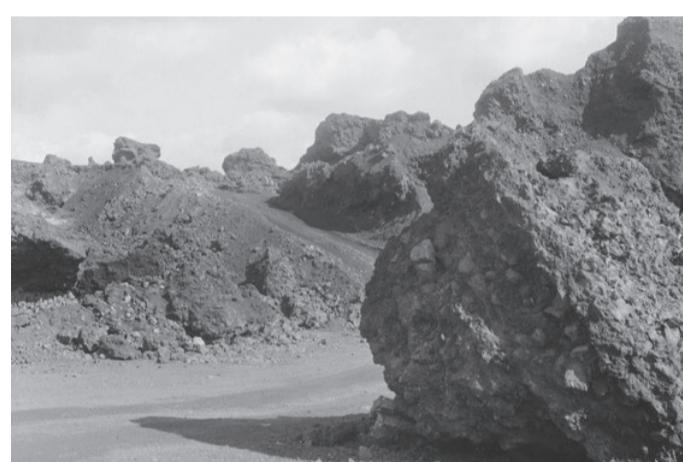
**9.** View of the slag tips to the north of the works site. The old copper smelting process produced a lot of iron-rich slag, which was initially just dumped.
