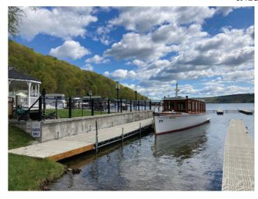
safer top-side travel for crew and to bring the passenger load closer to the center line for greater stability. Although the windshield is original, the deckhouse windows were replaced with safety glass. As the boat is powered with an ELCO electric motor, no fuel tank is needed.
