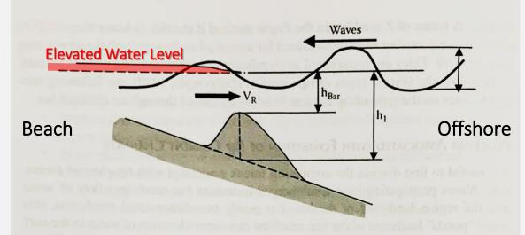
**FIGURE 6.1** Simple two-dimensional model for increased water level landward of the bar inducing a return flow velocity  $V_R$ . The  $h_1$  represents depth in the absence of the bar at the bar crest and was selected for illustrative purposes.
