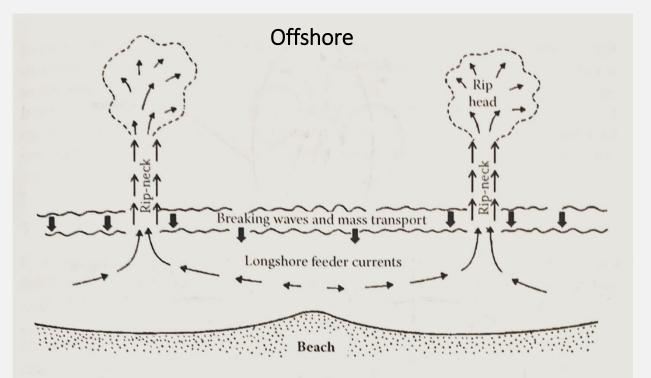
**FIGURE 1.2** Traditional paradigm of rip current circulation typically shows flow extending well beyond the surf zone. (*Source:* Modified from Komar, 1998. *Beach Processes and Sedimentation*, 2nd ed. Prentice Hall, New York.)
