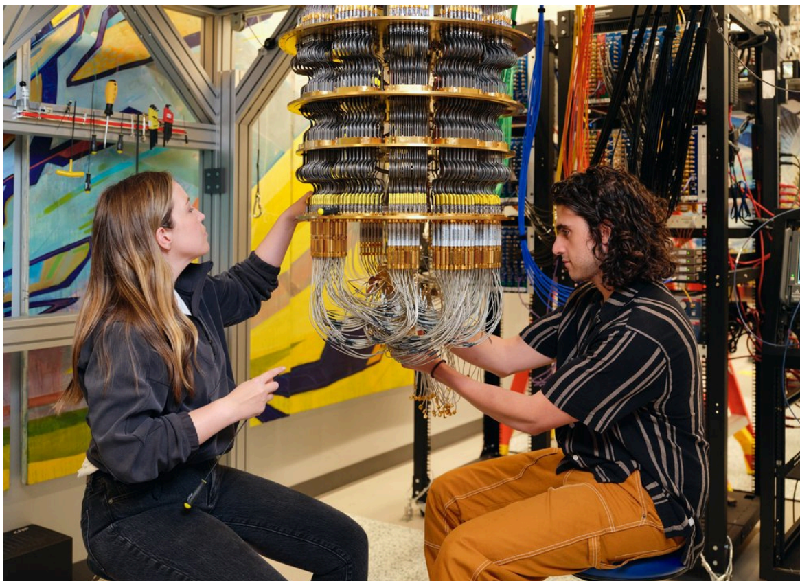
Google hardware technicians work on a quantum cryostat, a device that creates extremely cold environments for quantum computing calculations, at the tech giant's Quantum A1 research campus near Santa Barbara, California. (Google)
